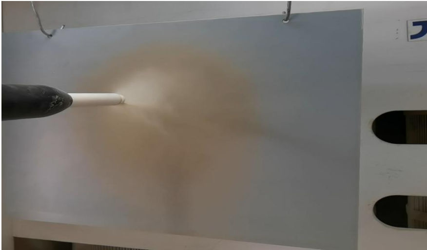
Most Powder Deposits on the Workpiece with Almost No Overspray
